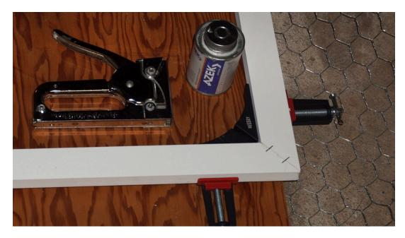
For the doors, I'm going to get fancy and make miter joints (at a 45 degree angle), because after all, I am using a miter saw! I'll secure the joints with glue and my trusty staple gun.
